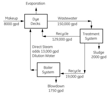
**Figure 1: Carpet Mill Approximate Water Balance After Recycling**
