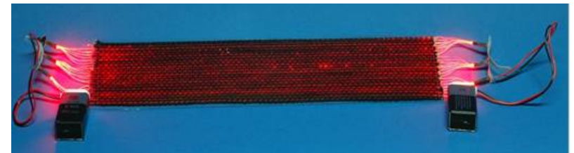
composite material with integrated optical fibres
