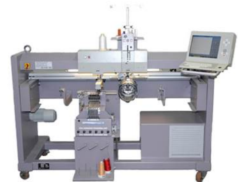
Embroidering machine with 3D-TFP fixation device and K-head for kettle and moss embroidering
