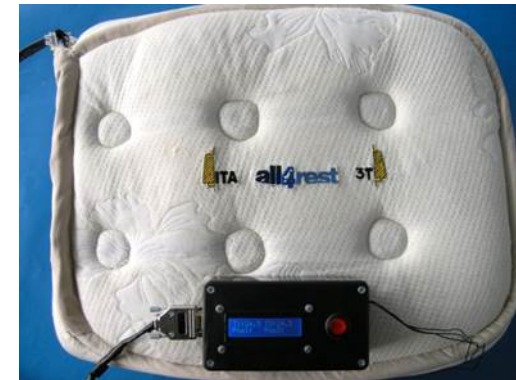
Prototype of mattress with temperature and movement sensor
