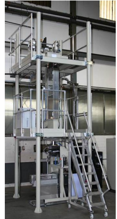
Biocomponent spinning plant
