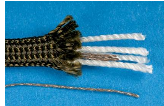
Sensor filament in a braided rope
