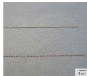
Embroidered platinum fibre for electro simulation
