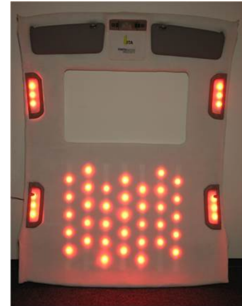
Roof interior with textile integrated LEDs
