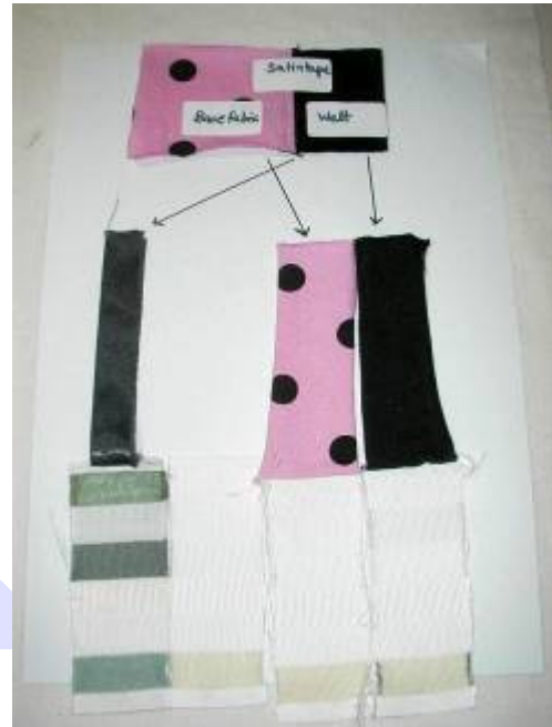
Tested specimens showing excellent colourfastness to washing of main fabrics but very poor fastness of the satin tape trim.
