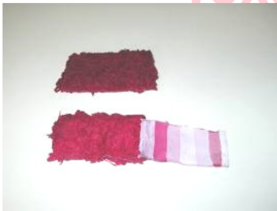
Sample of rug showing shade change and staining in the colourfastness to washing test.
