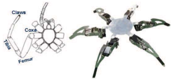
Fig 3 (Right side) Dorsal side of spider with proposed circular shape hexapod mechanical structure (Left side)
